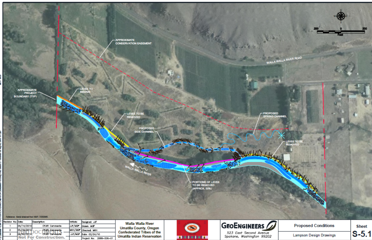
Figure 5: Restoration alternative (draft) for the Lampson project site on the mainstem Walla Walla River. The design includes, levee removal along most of the right bank, the construction of an 800' side channel designed to convey 10% of the flow, the placement of more than 200 whole conifer trees, placement of several hundred boulders, and improved shoreline slope.
