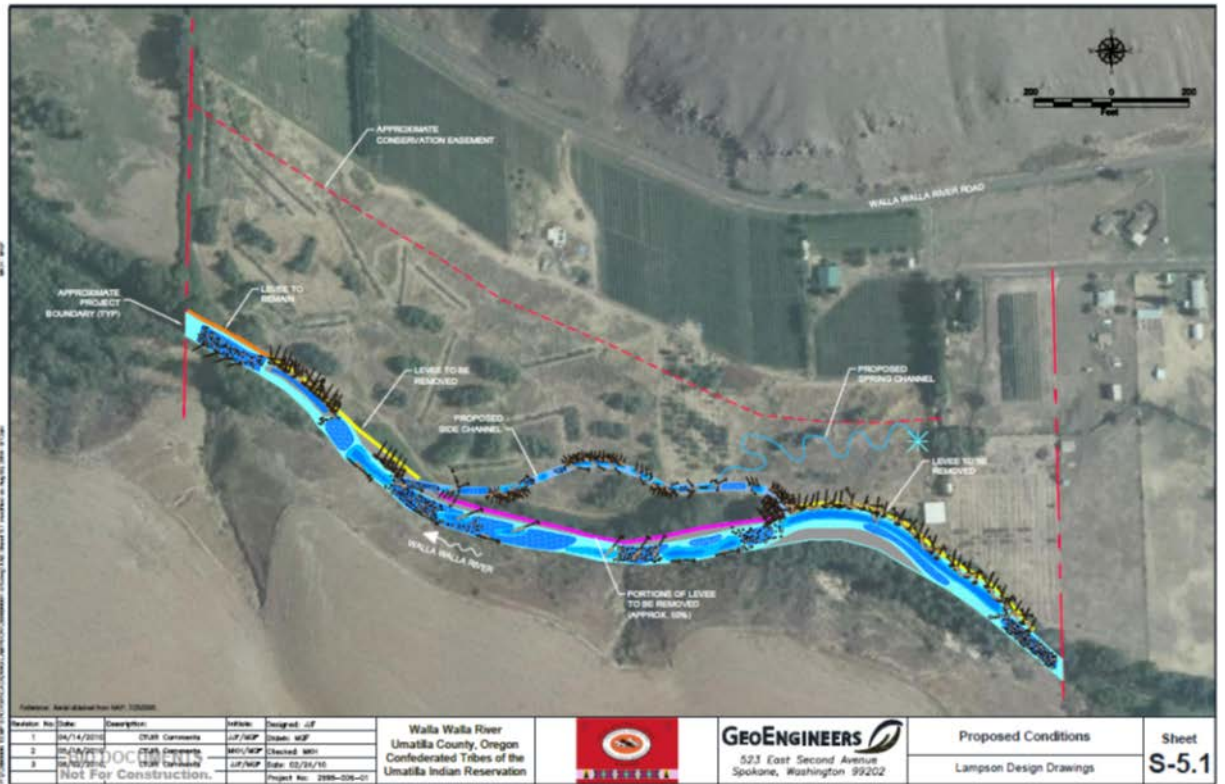
Figure 3: Restoration plan view for the Lampson project site on the mainstem Walla Walla River. The design includes levee removal along most of the right bank, the construction of a 600 meter side channel designed to convey 10% of the flow, the placement of more than 400 whole conifer trees, reconstructed floodplain, and improved riparian width and function.
