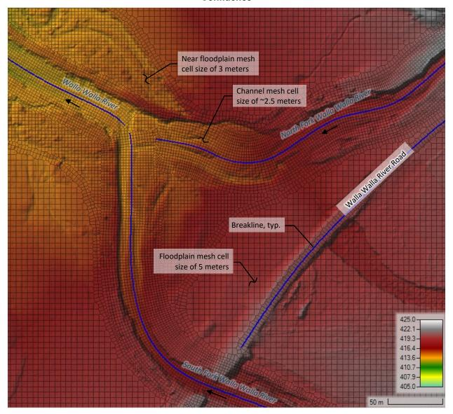
Figure 3: Post-flood Conditions Model Mesh at the North Fork and South Fork Walla Walla River
