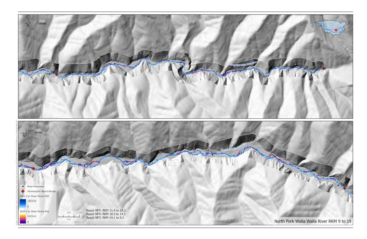
Figure 4-65. Shear stress of the 2-yr peak discharge for the 2019 and 2021 topobathymetric elevations of the NFWW River in reaches NF3, NF4, and NF5.
