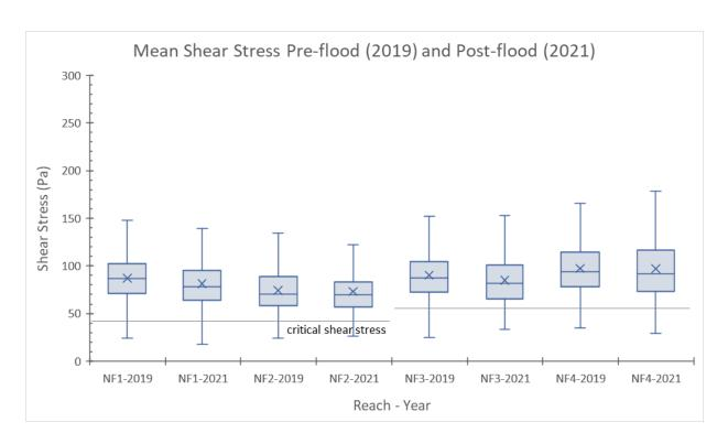
Figure 4-45. Mean shear stress for the 50% annual chance flood (2-yr peak) in the NFWW River.
