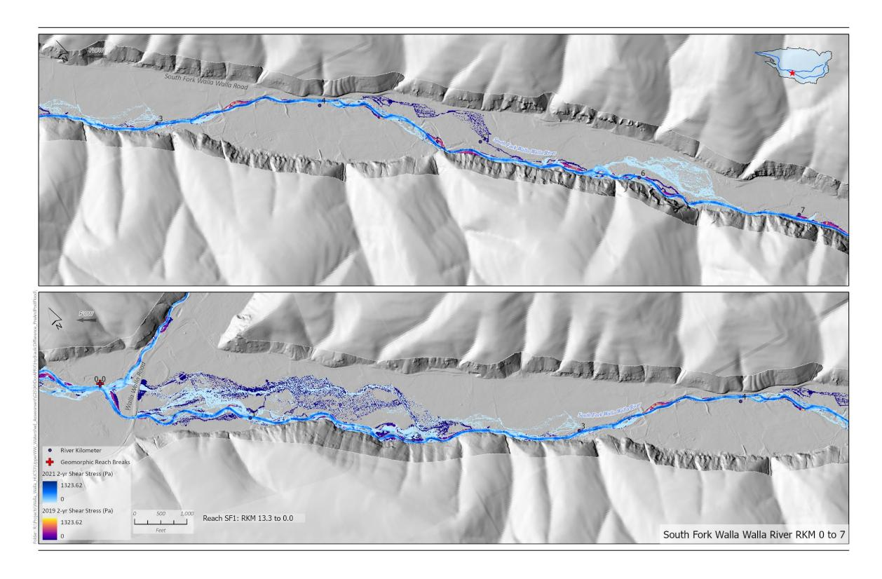
Figure 4-99. Shear stress of the 2-yr peak discharge for the 2019 and 2021 topobathymetric elevations of the SFWW River in reach SF1.
