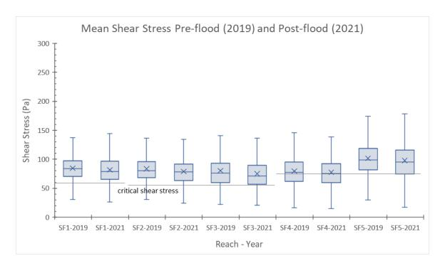
Figure 4-74. Mean shear stress for the 50% annual chance flood (2-yr peak) in the SFWW River.
