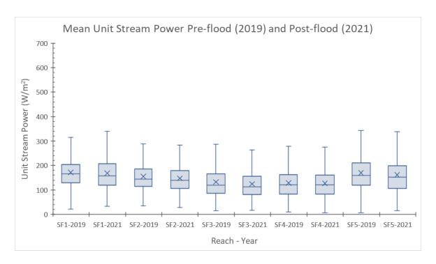
Figure 4-72. Mean unit stream power for the 50% annual chance flood (2-yr peak) in the SFWW River.
