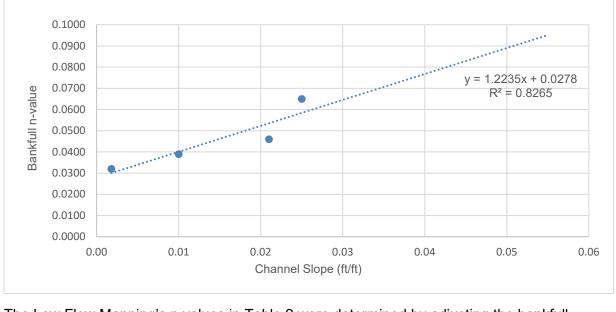
Figure 1: Channel Slope vs. Manning's n Regression for Bankfull Flows and Higher
