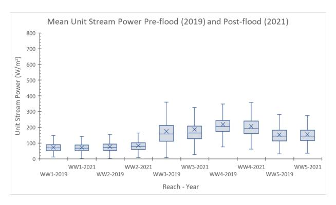
Figure 4-6. Mean unit stream power for the 50% annual chance flood (2-yr peak) in the WW River.
