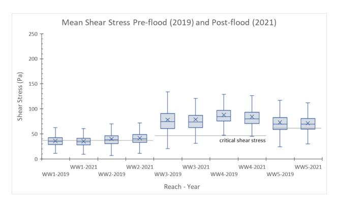
Figure 4-8. Mean shear stress for the 50% annual chance flood (2-yr peak) in the WW River.
