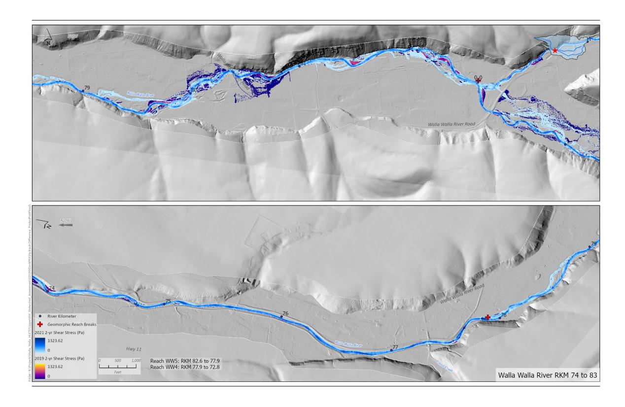
Figure 4-34. Shear stress of the 2-yr peak discharge for the 2019 and 2021 topobathymetric elevations of the WW River in reaches WW4 and WW5.
