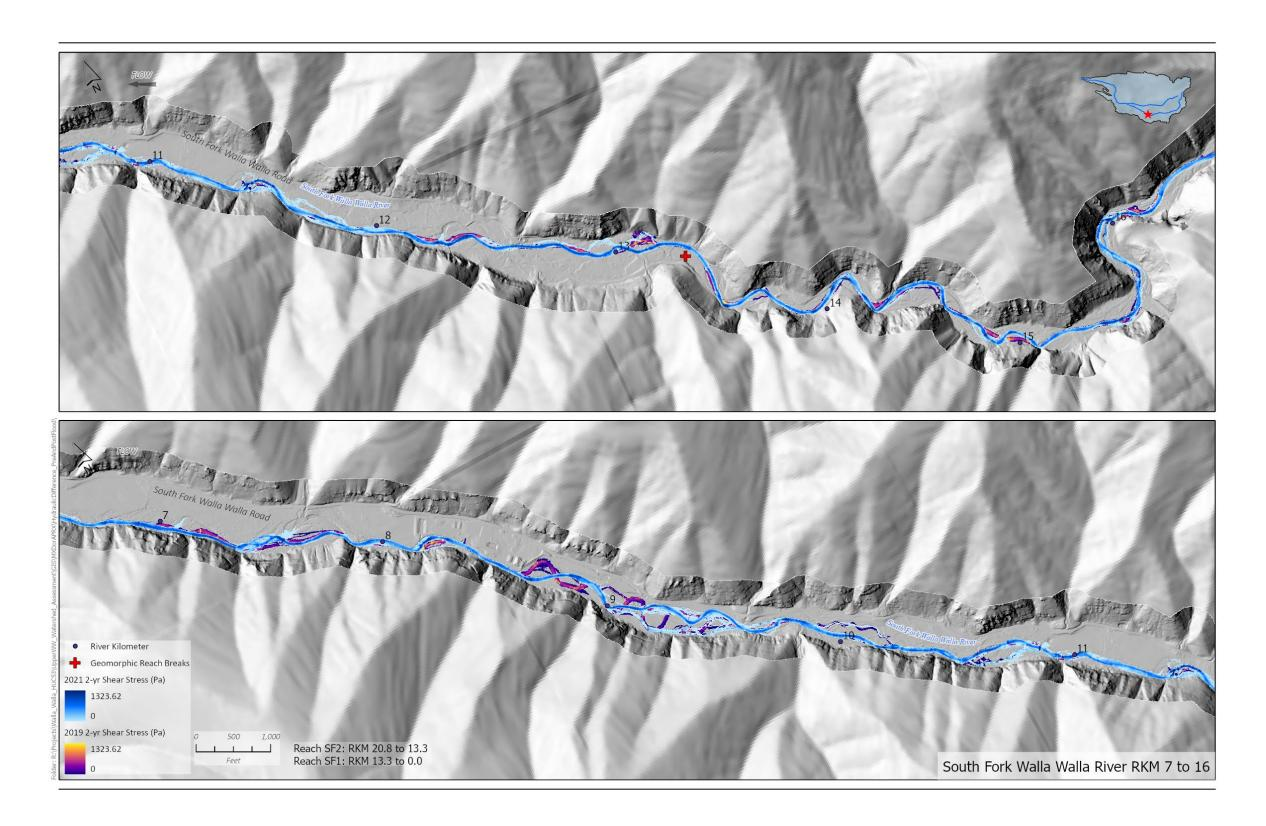
Figure 4-100. Shear stress of the 2-yr peak discharge for the 2019 and 2021 topobathymetric elevations of the SFWW River in reaches SF1 and SF2.
