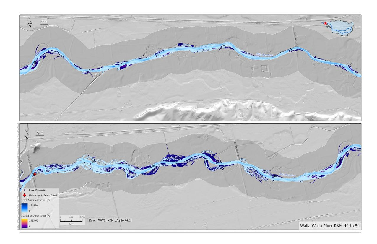
Figure 4-31. Shear stress of the 2-yr peak discharge for the 2019 and 2021 topobathymetric elevations of the WW River in reach WW1.
