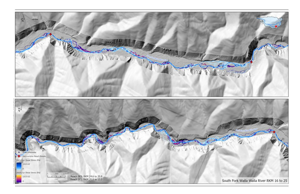
Figure 4-101. Shear stress of the 2-yr peak discharge for the 2019 and 2021 topobathymetric elevations of the SFWW River in reaches SF2 and SF3.
