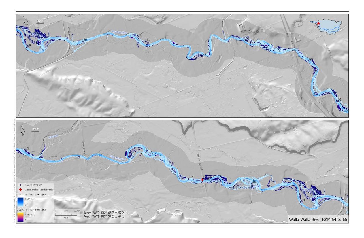
Figure 4-32. Shear stress of the 2-yr peak discharge for the 2019 and 2021 topobathymetric elevations of the WW River in reaches WW1 and WW2.
