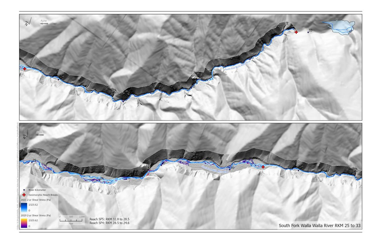
Figure 4-102. Shear stress of the 2-yr peak discharge for the 2019 and 2021 topobathymetric elevations of the SFWW River in reaches SF4 and SF5.
