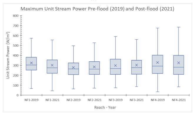
Figure 4-42. Maximum unit stream power for the 50% annual chance flood (2-yr peak) in the NFWW River.
