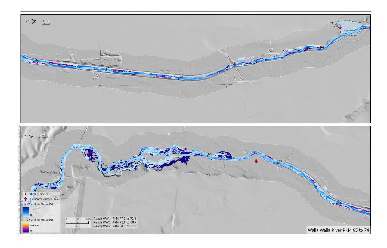
Figure 4-33. Shear stress of the 2-yr peak discharge for the 2019 and 2021 topobathymetric elevations of the WW River in reaches WW2, WW3, and WW4.
