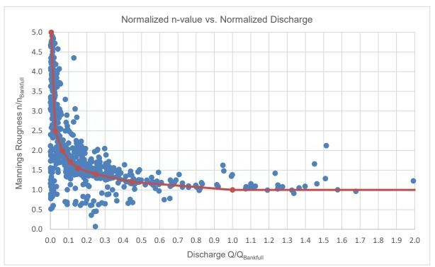
Figure 2: Q/Qbankfull vs. Manning's n/Manning's nbankfull Based on USGS Stream Gaging Stations
