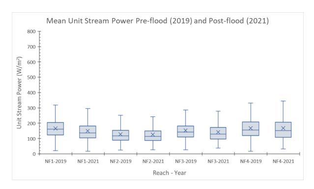
Figure 4-43. Mean unit stream power for the 50% annual chance flood (2-yr peak) in the NFWW River.
