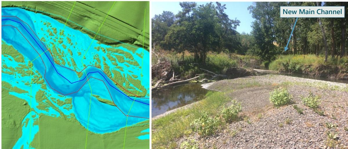
Left: The channel flows from right (upstream) to left (downstream) in this image. The annotated river centerline in dark blue traces the new path of the river through a narrow right channel resulting from a recent neck avulsion. However, the modeled river depth indicates the left channel is the main channel. Right: During the field visit, the view from upstream of the avulsion looking downstream shows the new narrow main channel on river right.
