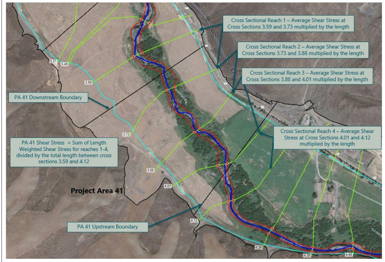
The average energy grade slope was calculated using the same array of cross sections, all of those that fall within the project area, as well as the cross sections immediately upstream and downstream. The energy grade elevation at each cross section at the upstream and downstream ends of the project area was differenced and divided by the total length to determine the energy grade slope for the project area.
