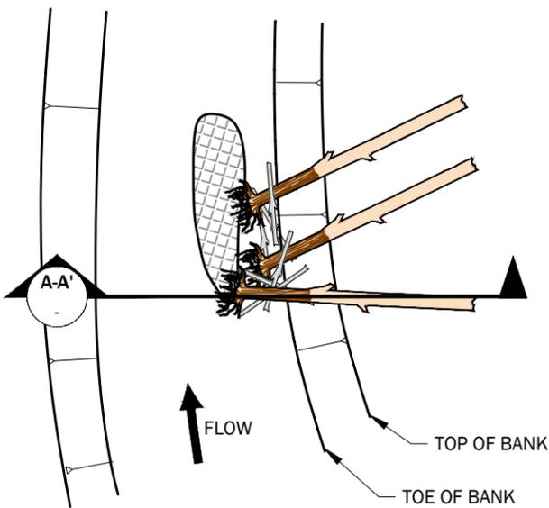
LOG ORIENTATION VARIES PER PLAN OR AS DIRECTED BY HYDRAULIC ENGINEER
