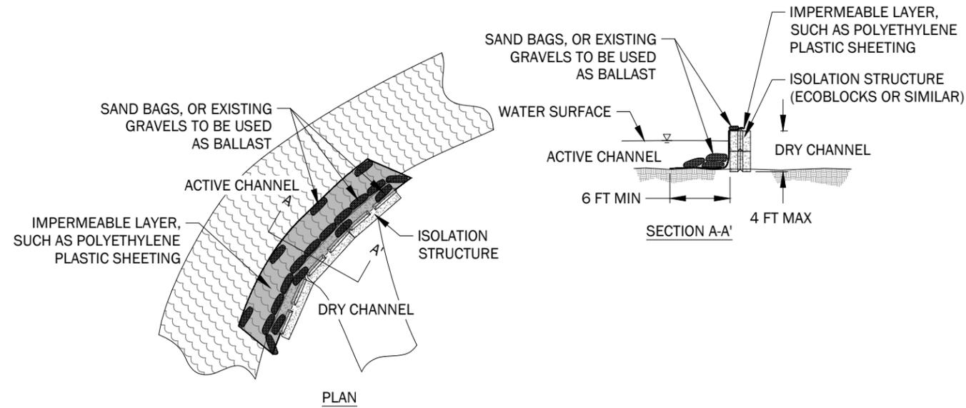
**SIDE CHANNEL WORK ZONE ISOLATION STRUCTURE** 1
