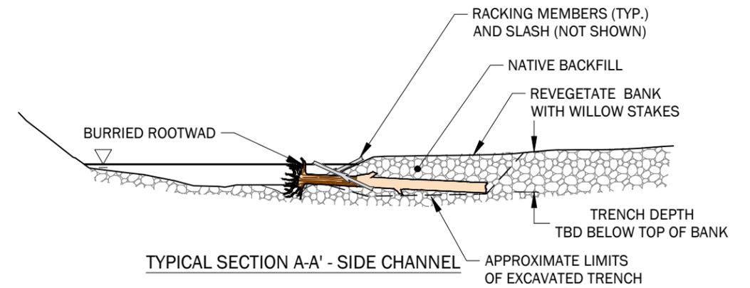
TYPICAL SECTION A-A' - SIDE CHANNEL
