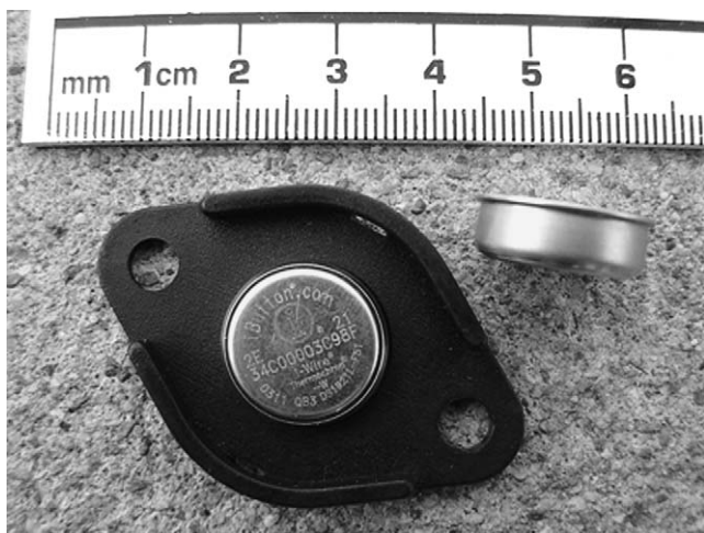
Figure 1. iButtons with mounting bracket. Unique identification code is stamped onto top of stainless steel housing. Side view is on the right.
