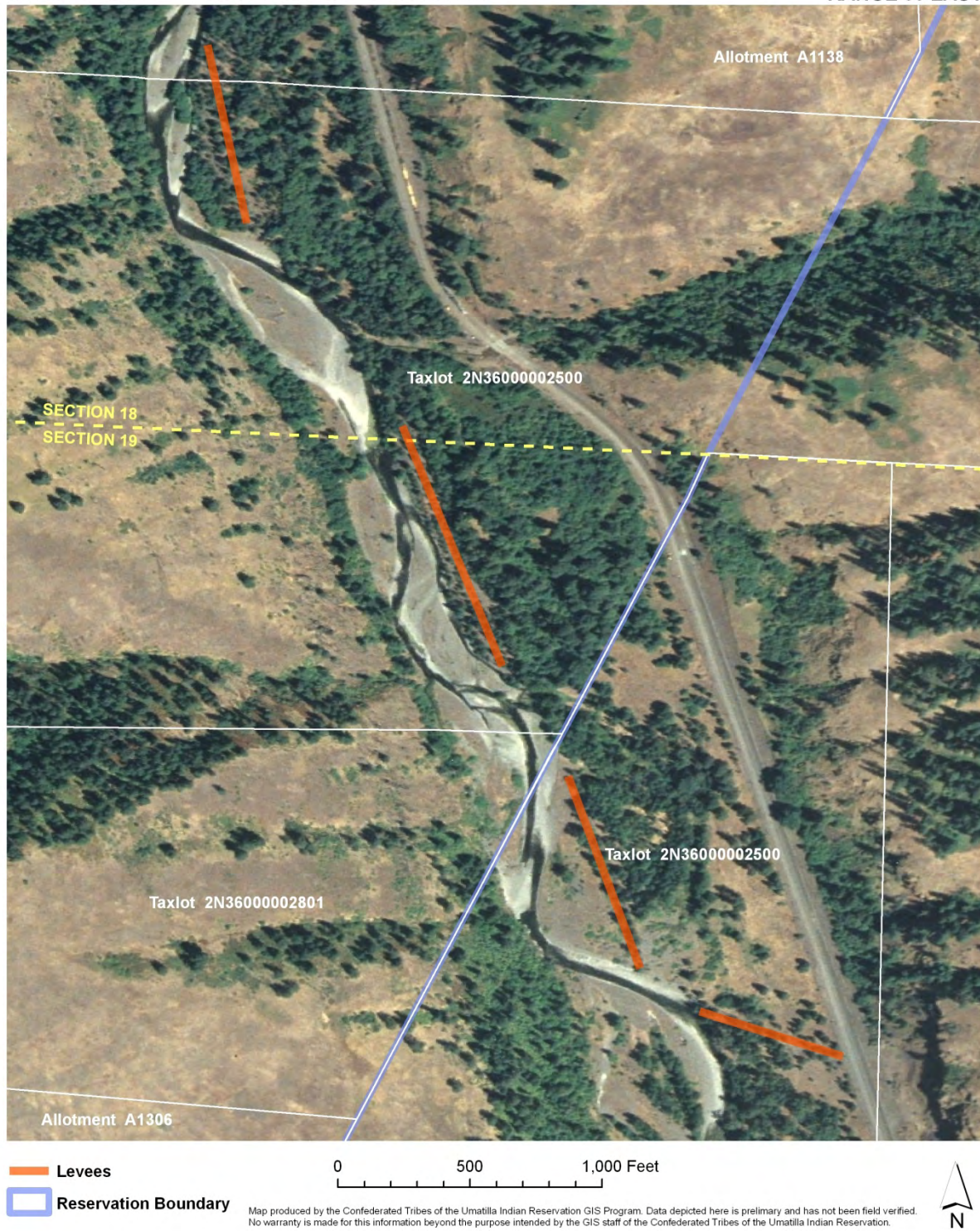
Figure 17. Identified Levees (Red) for Removal or Modification as Part of the Meacham Creek Levee Removal Project, RM's 5.0-6.0.
