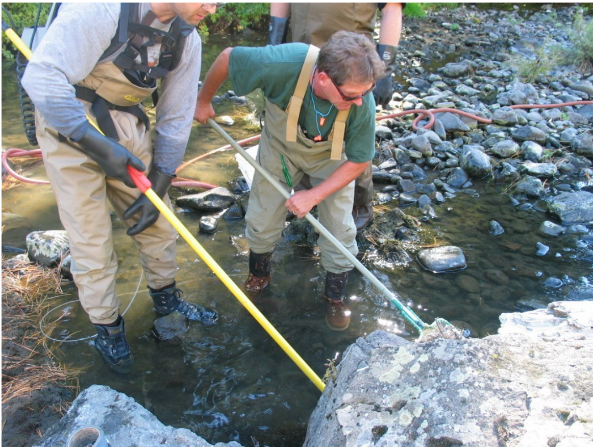
Figure 15. Methodology Used For Fish Population Monitoring Using Stream Electrofishers to Capture Salmonids at Project Sites Prior To Implementation
