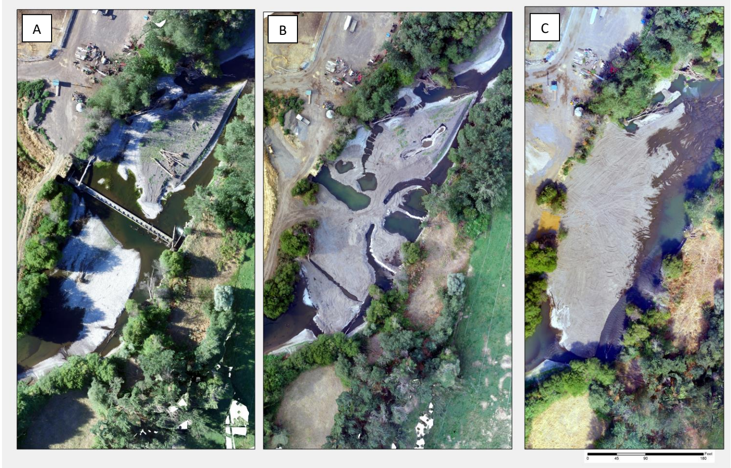
Figure 8. Drone imagery of the Dillon Dam Removal Project before (A), during (B), and after implementation (C).
