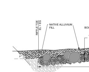
EMBED 24" AND 26" PLACE BOULDERS, BOULDERS IN FG PER CAR FILL VOIDS WITH STREAMBED GRAVELS, SEE TABLE FOR D50 APPROX KEY IN ROCK 4' BELOW THICK CREST APPROX 40 FT PROFILE A-A'
