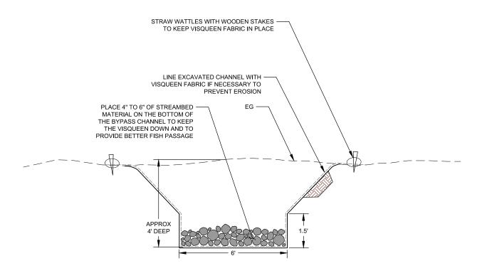
VISQUEEN TEMP BYPASS CHANNEL TYPICAL SECTION
