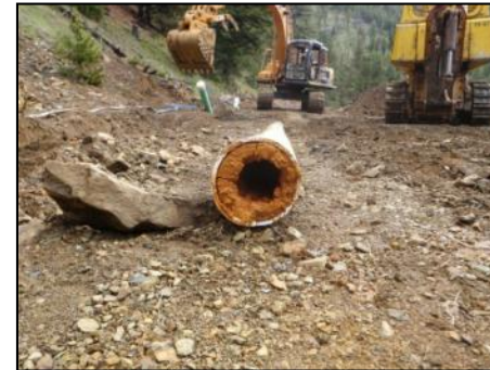
Old Red Boy Mine pipeline partially clogged by precipitates (above) and new line (right)
