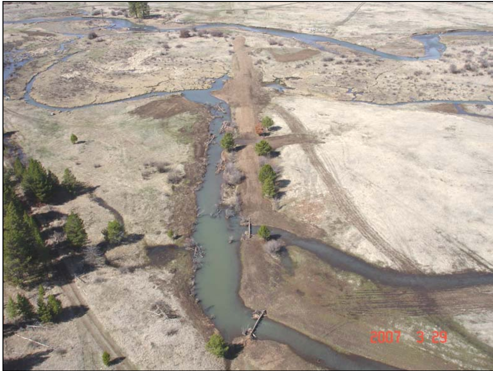
March 2007, Meadow Creek Restoration Project – Photo illustrates pond manifold developed by taking advantage of an old highway road prism. Manifold is utilized as a water control structure to manage streamflow into wetland restoration network.
