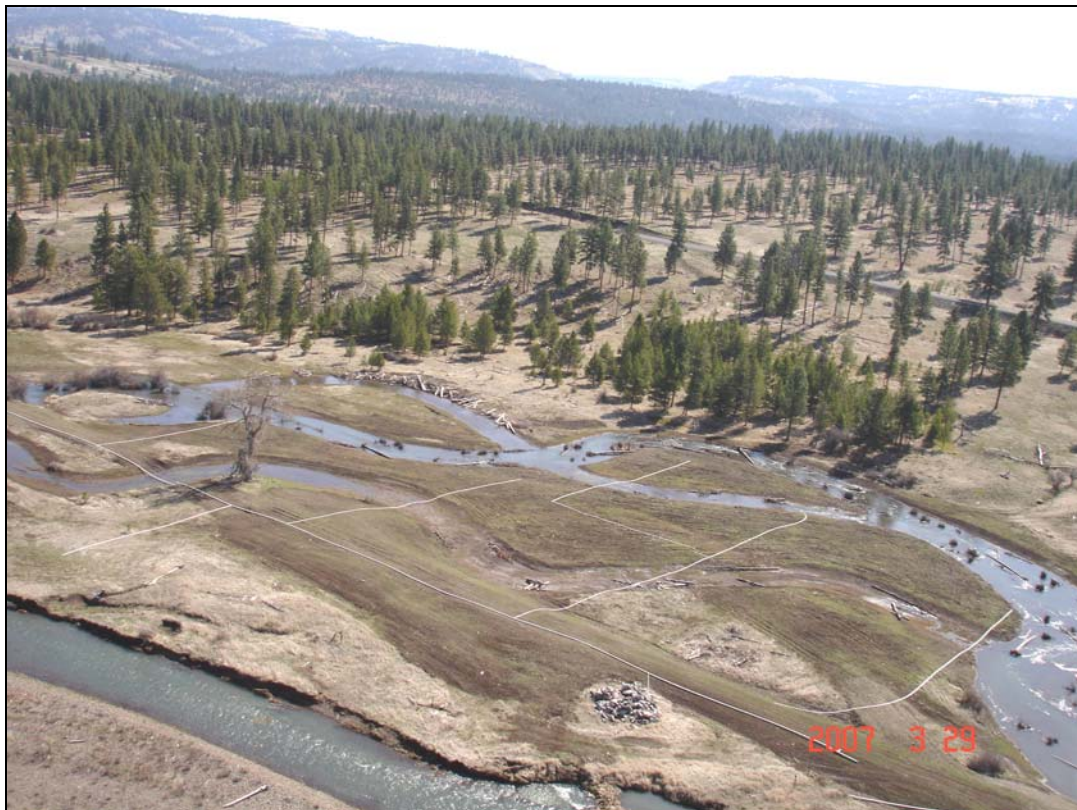
March 2007, Meadow Creek Restoration Project – Photo illustrates upper project area during spring high flow conditions. Note temporary irrigation system installed during summer 2006 to facilitate vegetative recovery.
