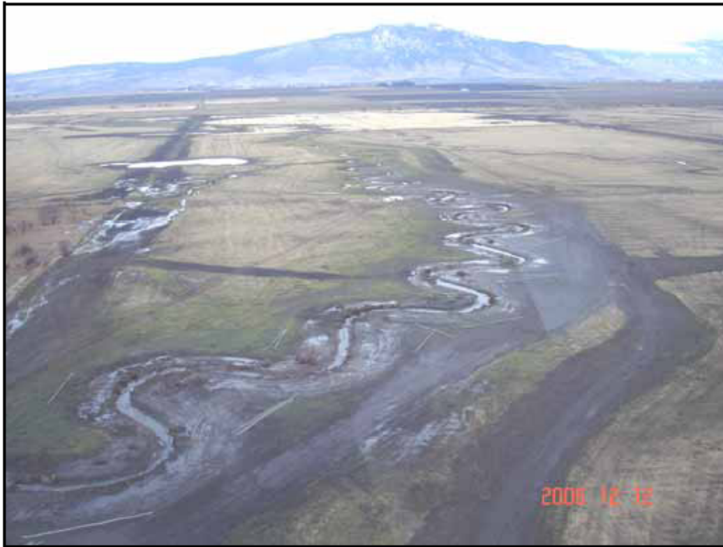
Upstream reach of End Creek (Rice) Restoration Channel, viewing east (downstream) towards South Fork Willow Creek confluence. Note reclaimed channelized reach in left corner of photo and floodplain ponds incorporated into reclamation plan. December 2006
