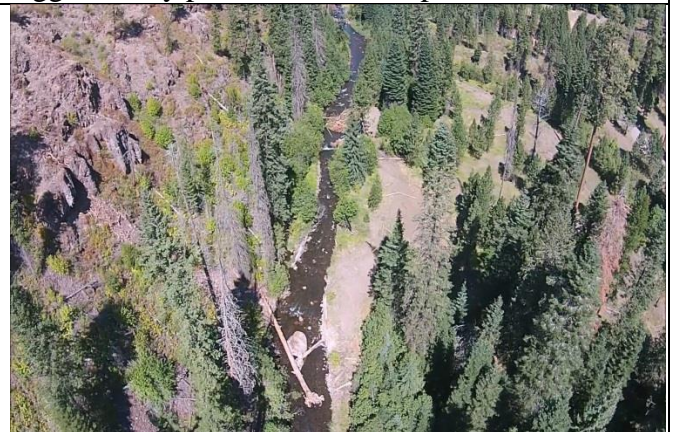
Aggressively placed root wads; pool formation
