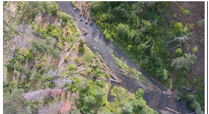
Aggressively placed root wads; pool formation
