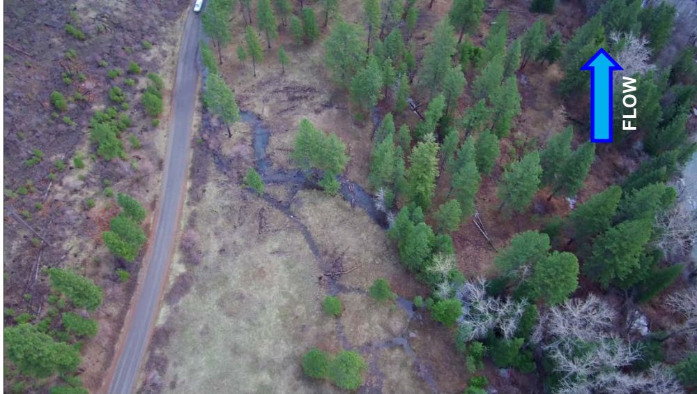
Figure 25: Imagery of PA3 floodplain inundation on April 10, 2019. Imagery was acquired by the CTUIR drone program. Discharge was estimated to be ~400-600 cfs within the reach. These estimates were derived from USGS Stream Stats and regression models developed by design engineers (Tetra Tech, 2014).
