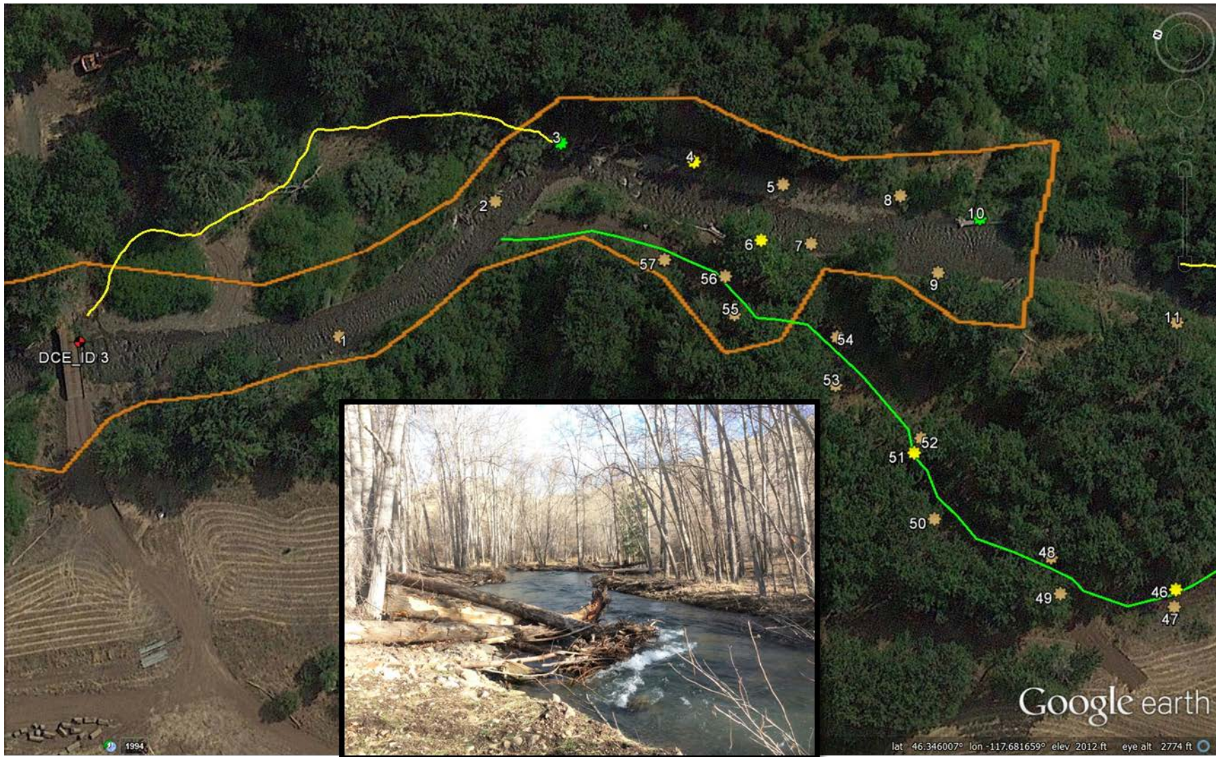
Figure 23: Project Area 15, Tucannon River channel complexity and connectivity project completed by the Columbia Conservation District in August 2014. The Google Map illustrates the placement point for structures natural and placed measured in the rapid habitat survey. The green icons show natural wood, yellow placed unanchored wood and the brown anchored placed wood. The green line indicates the new channel delineation and the yellow side channel is an existing high flow channel modified during the project. The inset shows the lower end of the new channels during 130 cfs event.
