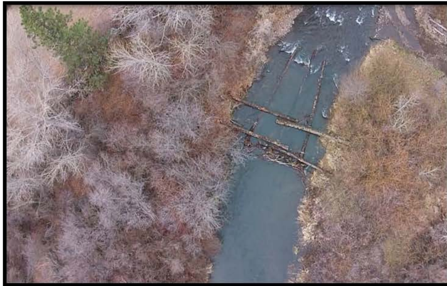
Figure 22: Project Area 15, Tucannon River channel complexity and connectivity project completed by the Columbia Conservation District in August 2014. (Upper) The left and right photos are of the same location at different perspectives. Note the left image has the temporary bridge placed at the existing ford during construction. (Lower) Left image is of the channel spanner placed to aggrade the stream bed and capture wood during elevated flow in December 2014. Right image shows the backwatered pool and confluence of the two channels.
