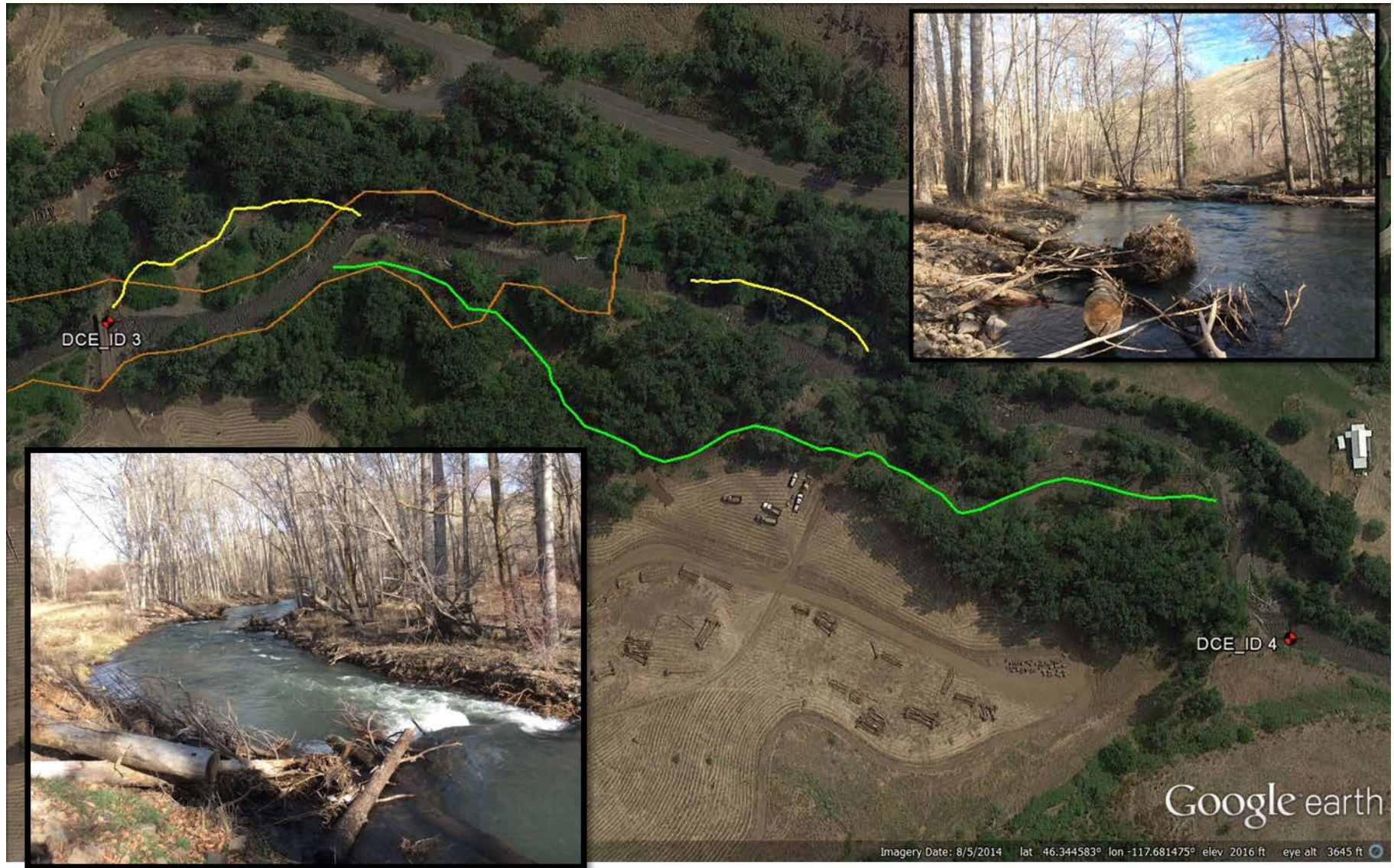
Figure 24: Figure 23: Project Area 15, Tucannon River channel complexity and connectivity project completed by the Columbia Conservation District in August 2014. The Google Map illustrates the position of the side channels created (green) or augmented (yellow) under this project. The two insets were taken in the created side channel during 250 cfs event in February 2015.
