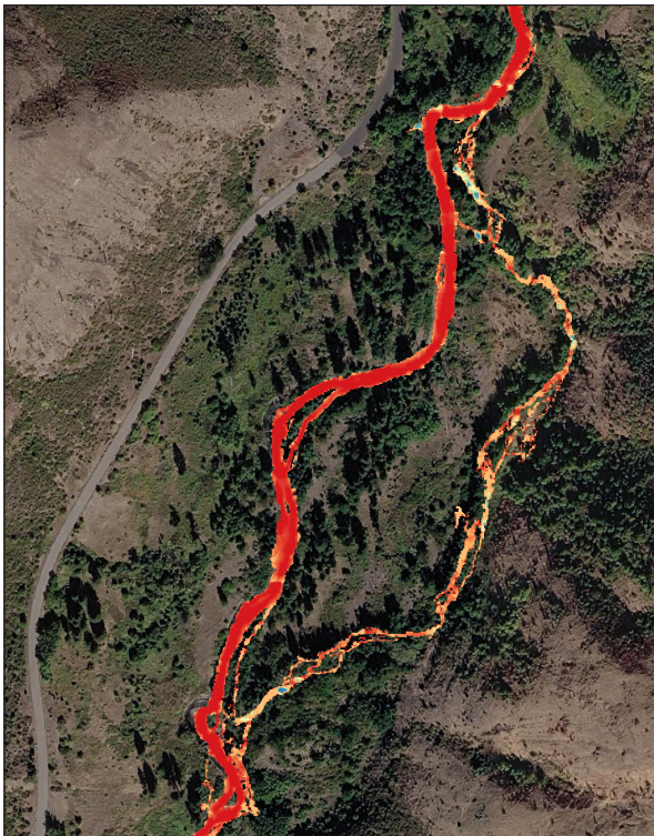
■ Figure 21. Single and multi-thread channel complexes with relatively high habitat suitability. Exchange, channel migration, and the development of multi-thread channels, side channels, alcoves, pools, and other complex channel features create slower, deeper hydraulic environments that are more suitable for multiple juvenile life stages.
