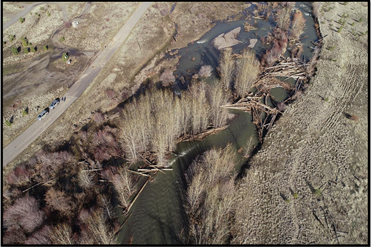
Figure 7: Example of large post 2020 flood log jam complex created by mobile LWD transported downstream from PA11.1 to form the large jam complex in PA11.2.
