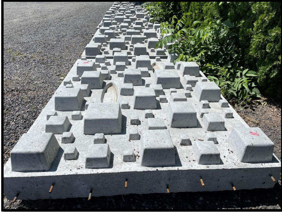
Figure 25: Fish way roughness panel purchased with BPA contract (#86820) in 2022.
