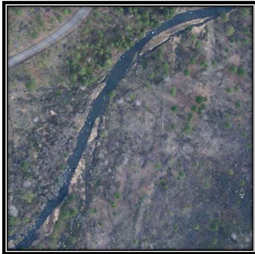
Figure 5: Tucannon River Project Area 10 April 2010 pre project photo of sample reach to be treated with LWD augmentation. Existing condition in this reach exhibited plain bed channel with almost no existing LWD Key pieces.
