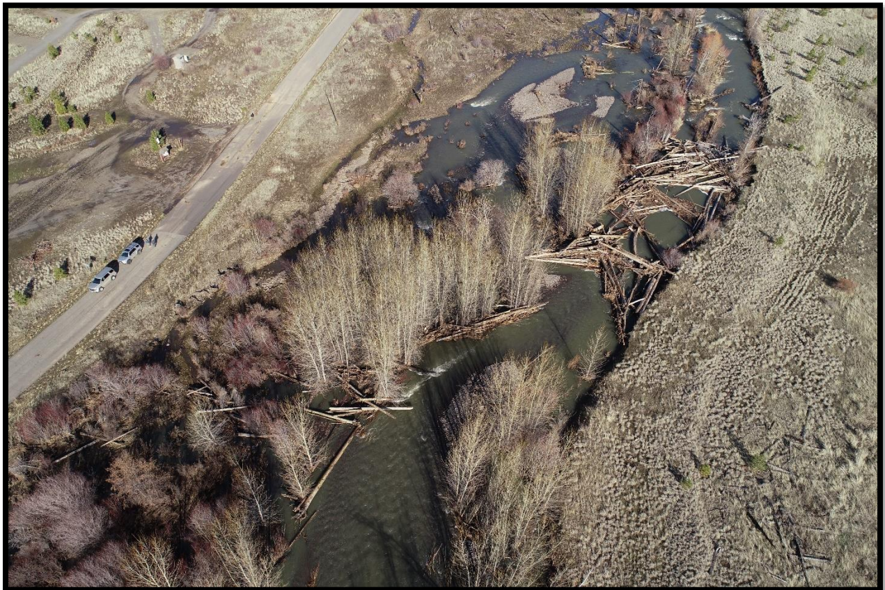
Figure 5: Example of large post 2020 flood log jam complex created by mobile LWD transported downstream from PA11.1 to form the large jam complex in PA11.2.
