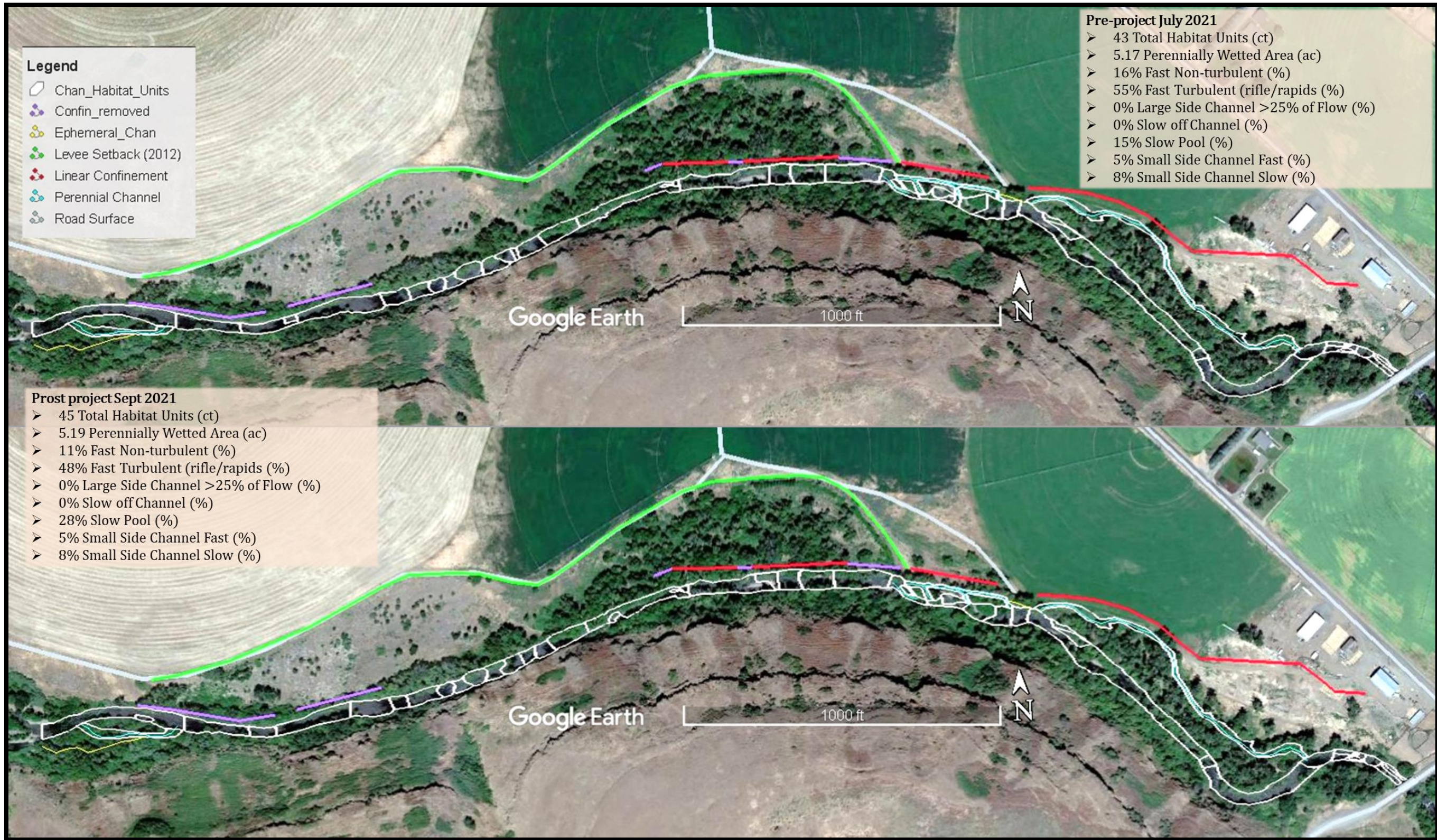
Figure 28: Project Area 26 (Phase II) channel habitats units delineated during the pre-project survey in July 2021 and the as-built survey September 2021. The greatest immediate changes in habitat units were in conversion of riffle/rapid units to slow water pools and non-turbulent glides.
